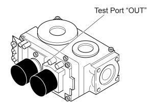
Figure 10 - Pressure Test Point Location
